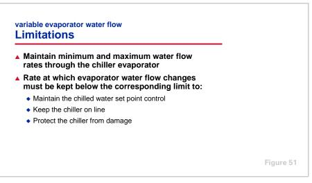
The controls on many current chiller designs can properly control the chiller in response to varying evaporator flow rates, with the following limitations:
